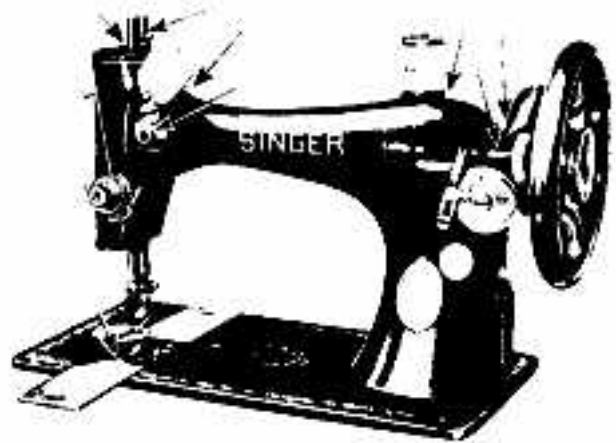
FIG. 16. OILING POINTS AT THE FRONT OF THE MACHINE
